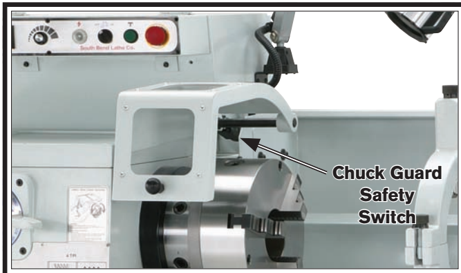
Figure 150. Chuck guard limit switch.
